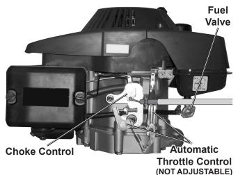
**Fuel Valve** - This controls the fuel supply to the engine.
